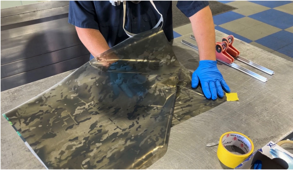
Image 1 How to Peel Clear Backing from Film
